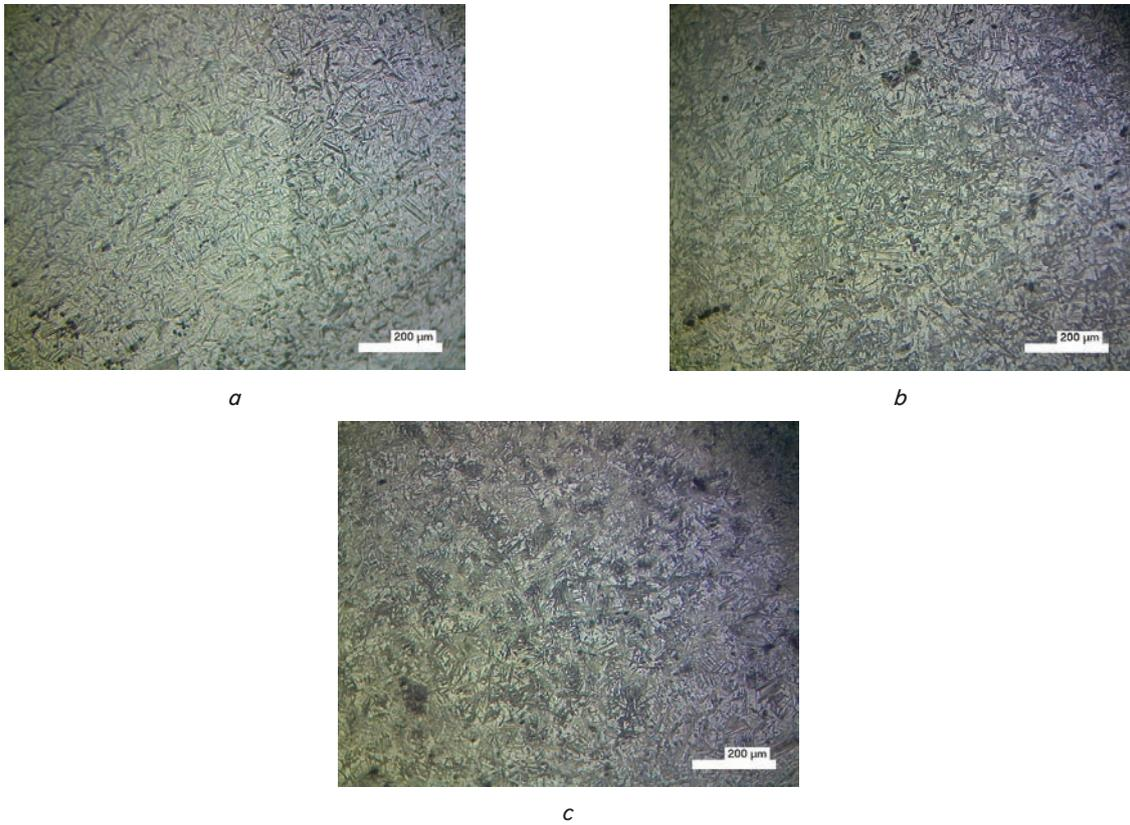
Fig. 5. Cross-sectional microstructure of the specimen using coil code *B*: *a* – fine martensite structure on the upper side; *b* – fine tends to be coarser martensite structure on the middle side; *c* – coarse martensite structure on the lower side
