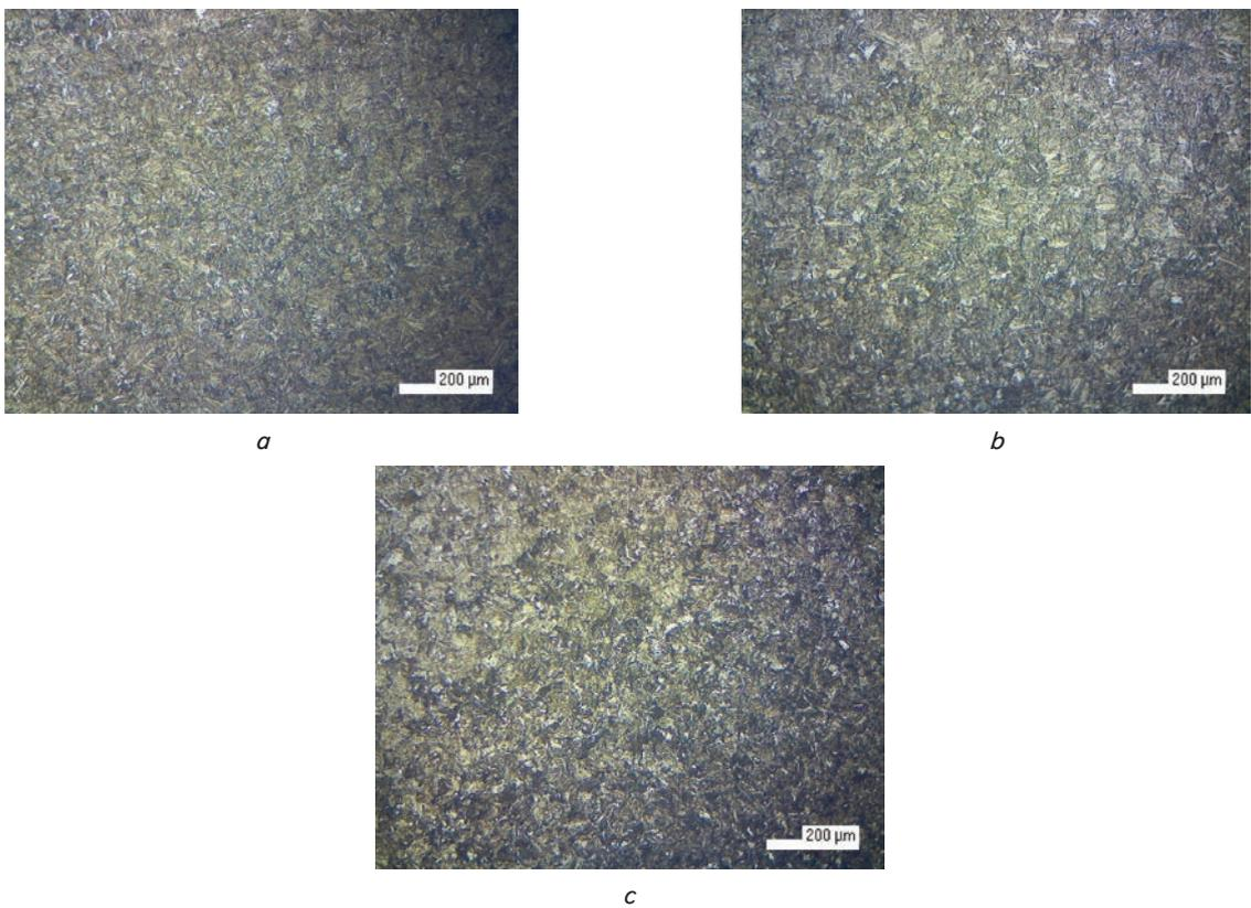
Fig. 6. Cross-sectional microstructure of the specimen using coil code *C*: *a* – fine martensite structure on the upper side; *b* – fine martensite structure on the middle side; *c* – fine martensite structure on the lower side
