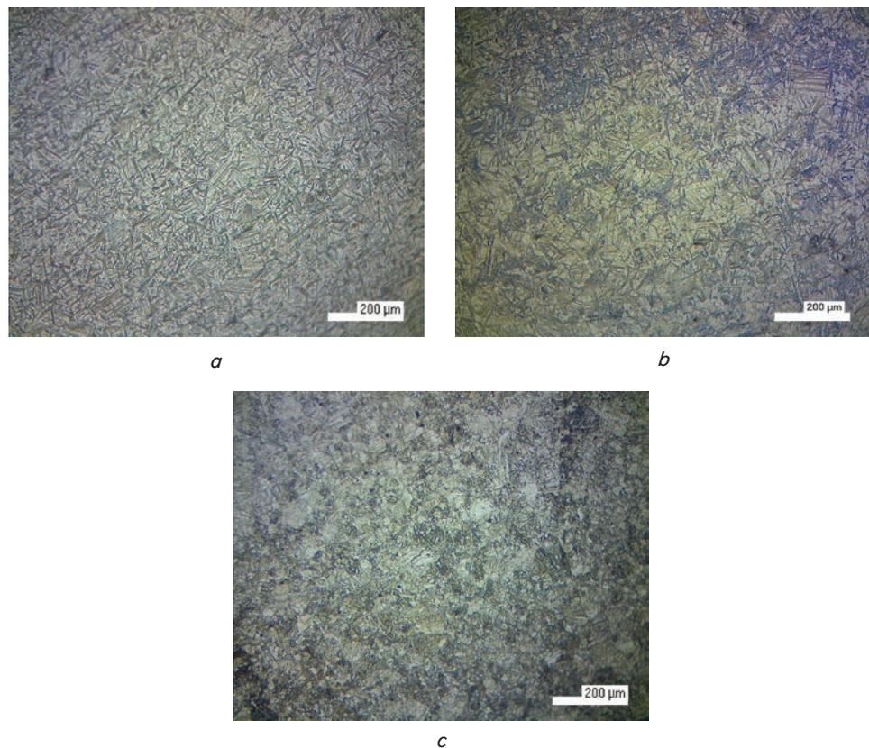
Fig. 4. Cross-sectional microstructure of the specimen using coil code *A*: *a* – fine martensite structure on the upper side; *b* – coarse martensite structure on the middle side; *c* – coarse martensite and some of the remaining perlite and ferrite structure on the lower side
