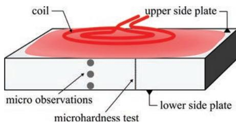
Fig. 2. Specimens for microstructure and microhardness tests
