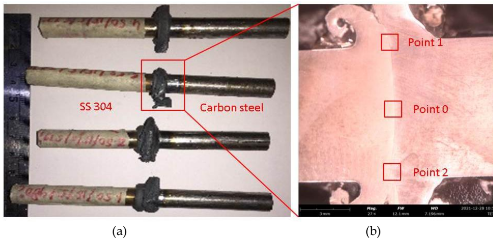
Figure 1: Friction welding results a). joint and b). cross-section of the joint
