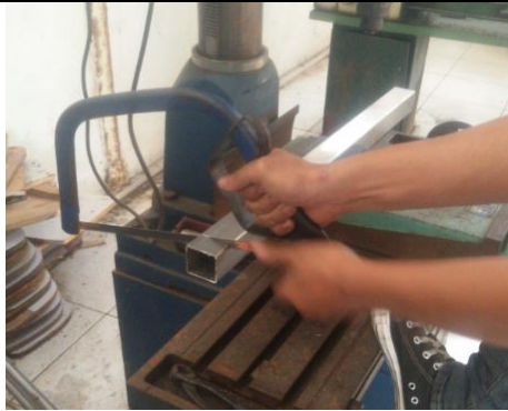
Proses pemotongan material stainless steel hollow 304
