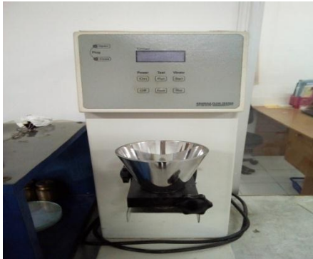
Granul Flow Tester ( GFT-100-AU-PN )
