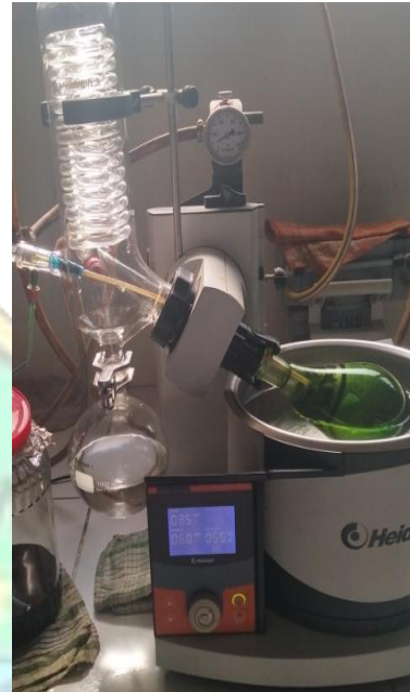
Proses rotari evaporator daun
